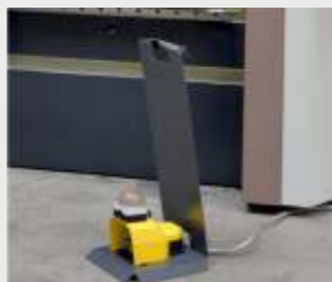
Foot Pedal with Emergency Stop Button
